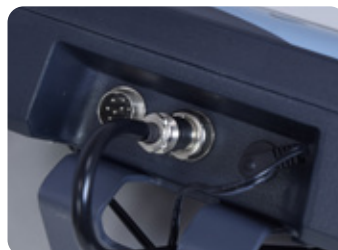
Platform indicator and power supply connection. Wall or overground support
