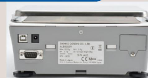
RS232C and USB are installed as standard to connect to outside devices like PC and printer. Extension RS232C, ethernet and relay contact can be available as additional option.
