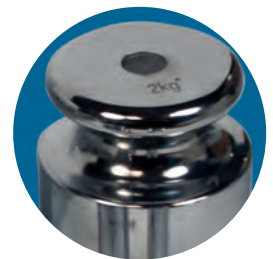
Top adjustment cavity
