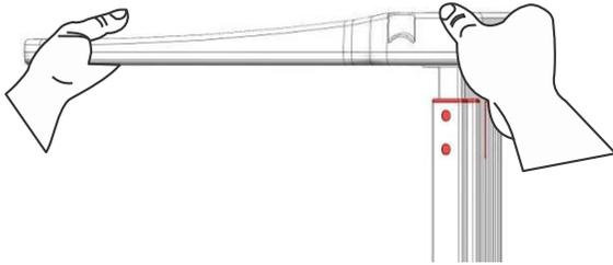
1. Place both hands in place as figure to hold the height rod's head.
