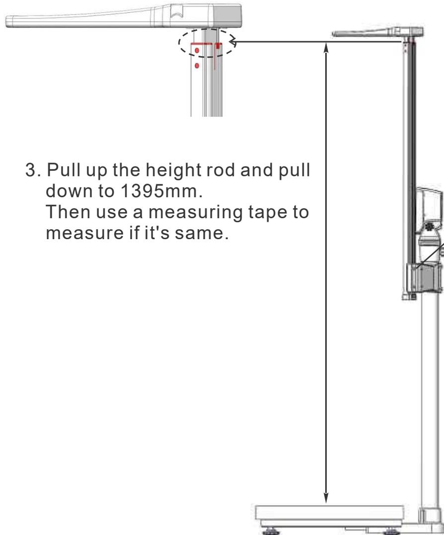
3. Pull up the height rod and pull down to 1395mm. Then use a measuring tape to measure if it's same.
