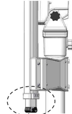
Note: If the inner height rod slide down easily, you could adjust the screw.
